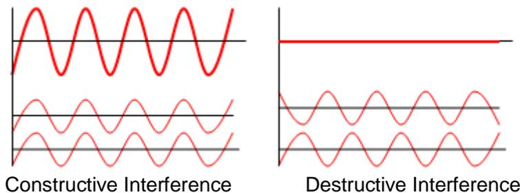
This process is called interference, and the device that does it is called an interferometer. (if you have a special interest in this technology, ask receptionist to view the movie).
