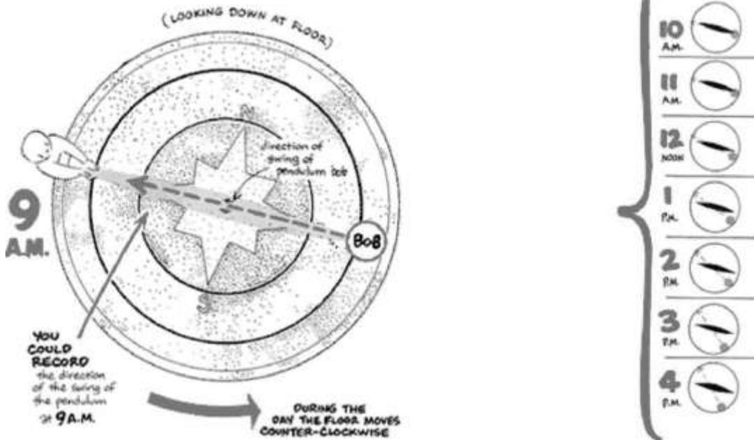
At Perth latitude, the floor turns **about 220°** under the pendulum in **about 24 hours** (at South Pole, it would turn a full circle 360°).
